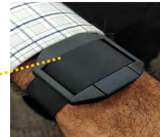
MotionSense HRV: accelerometers, gyroscopes, PPG
